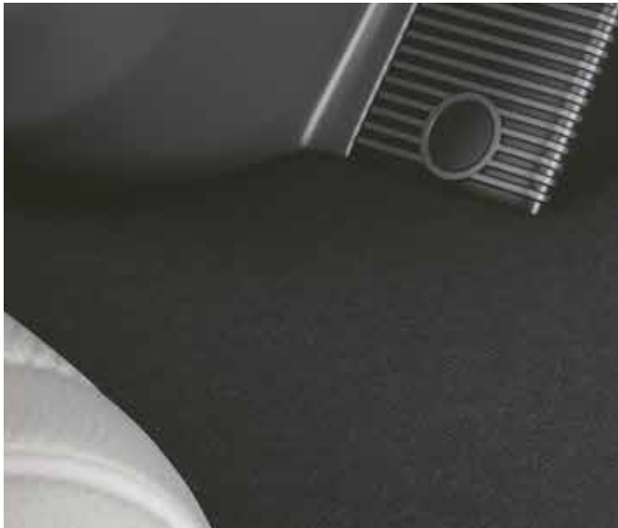
The headlining and carpet fabric includes bio components extracted from sugarcane and corn.
