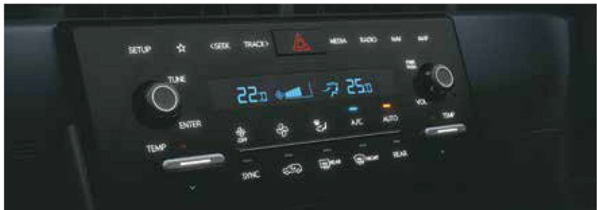
Dual zone automatic temperature control (DATC) with touch control
