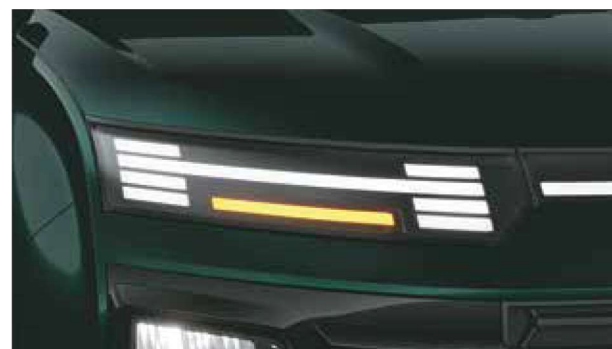
LED turn signal with sequential function
