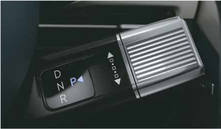
Shift by wire (SBW Column type)
