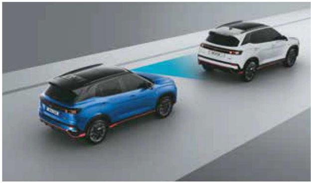
Forward Collision - Avoidance Assist - Car (FCA-Car) & Forward Collision Warning (FCW)
