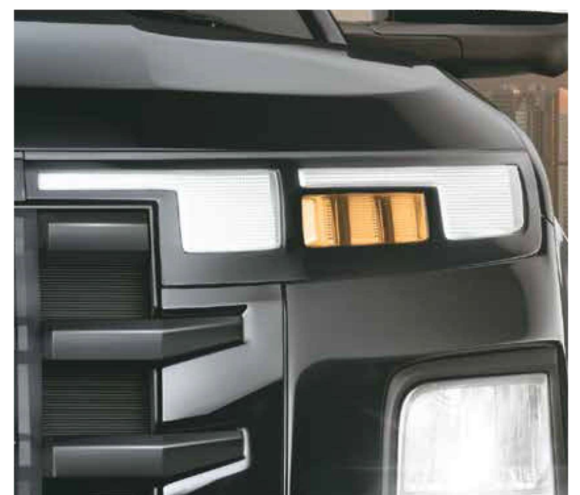
Front turn signal with sequential function
