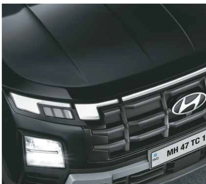
Horizon LED positioning lamps & DRLs
